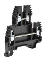
Konnect-It screw double-level feedthrough terminal block, accepts wire size 26-12 AWG, black, 20A, 35mm DIN rail mount, 100kA SCCR. Package of 25. For use with jumpers KN-2J12, KN-3J12, KN-4J12 and KN-10J12.
