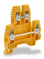
Konnect-It screw double-level feedthrough terminal block, accepts wire size 26-10 AWG, yellow, 30A, 35mm DIN rail mount, 100kA SCCR. Package of 100. For use with jumpers KN-2J10, KN-3J10, KN-4J10 and KN-10J10.
