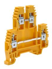
Konnect-It screw double-level feedthrough terminal block, accepts wire size 26-10 AWG, yellow, 30A, 35mm DIN rail mount, 100kA SCCR. Package of 25. For use with jumpers KN-2J10, KN-3J10, KN-4J10 and KN-10J10.
