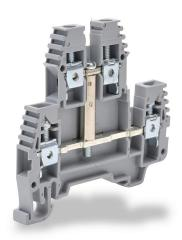
Konnect-It screw double-level feedthrough terminal block, connected between levels, accepts wire size 26-10 AWG, gray, 30A, 35mm DIN rail mount, 100kA SCCR. Package of 20. For use with jumpers KN-2J10, KN-3J10, KN-4J10 and KN-10J10.
