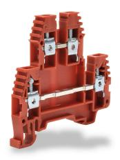
Konnect-It screw double-level feedthrough terminal block, accepts wire size 26-10 AWG, red, 30A, 35mm DIN rail mount, 100kA SCCR. Package of 100. For use with jumpers KN-2J10, KN-3J10, KN-4J10 and KN-10J10.
