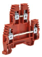
Konnect-It screw double-level feedthrough terminal block, accepts wire size 26-10 AWG, red, 30A, 35mm DIN rail mount, 100kA SCCR. Package of 25. For use with jumpers KN-2J10, KN-3J10, KN-4J10 and KN-10J10.
