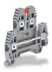
Konnect-It screw double-level feedthrough terminal block, connected between levels and power indicator, accepts wire size 26-10 AWG, gray, 30A, 24 VDC LED indicator(s), 35mm DIN rail mount, 100kA SCCR. Package of 20.
