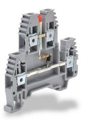
Konnect-It screw double-level feedthrough terminal block, connected between levels and power indicator, accepts wire size 26-10 AWG, gray, 30A, 24 VAC LED indicator(s), 35mm DIN rail mount, 100kA SCCR. Package of 20.
