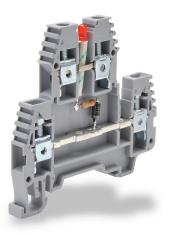
Konnect-It screw double-level feedthrough terminal block, connected between levels and power indicator, accepts wire size 26-10 AWG, gray, 30A, 110 VAC LED indicator(s), 35mm DIN rail mount, 100kA SCCR. Package of 20.
