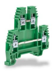
Konnect-It screw double-level feedthrough terminal block, accepts wire size 26-10 AWG, green, 30A, 35mm DIN rail mount, 100kA SCCR. Package of 100. For use with jumpers KN-2J10, KN-3J10, KN-4J10 and KN-10J10.
