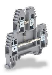
Konnect-It screw double-level feedthrough terminal block, connected between levels and diode, accepts wire size 26-10 AWG, gray, 30A, 35mm DIN rail mount, 100kA SCCR. Package of 20. For use with jumpers KN-2J10, KN-3J10, KN-4J10 and KN-10J10.
