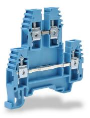
Konnect-It screw double-level feedthrough terminal block, accepts wire size 26-10 AWG, blue, 30A, 35mm DIN rail mount, 100kA SCCR. Package of 100. For use with jumpers KN-2J10, KN-3J10, KN-4J10 and KN-10J10.
