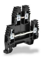
Konnect-It screw double-level feedthrough terminal block, accepts wire size 26-10 AWG, black, 30A, 35mm DIN rail mount, 100kA SCCR. Package of 100. For use with jumpers KN-2J10, KN-3J10, KN-4J10 and KN-10J10.
