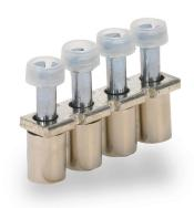
Konnect-It terminal block jumper, screw-down type, 4-pole, 32A, 750V. Package of 15. For use with KN-T10 or KN-D10 series block.
