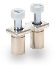
Konnect-It terminal block jumper, screw-down type, 2-pole, 41A, 630V. Package of 25. For use with KN-T8 series block.
