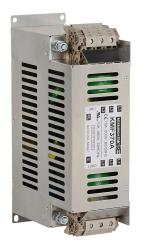
Roxburgh EMI input filter, 230/460 VAC, 3-phase, 70A, panel mount, EMI/RFI filtering, 2-stage, drive rated, high performance, screw terminals. For use with 3-phase AC drives.
