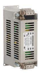
Roxburgh EMI input filter, 230/460 VAC, 3-phase, 50A, panel mount, EMI/RFI filtering, 2-stage, drive rated, high performance, screw terminals. For use with 3-phase AC drives.
