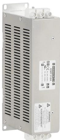
Roxburgh EMI input filter, 230/460 VAC, 3-phase, 18A, panel mount, EMI/RFI filtering, 2-stage, drive rated, high performance, screw terminals. For use with 3-phase AC drives.
