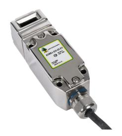
IDEM safety switch, tongue (key) interlock, hazardous location rated, 90-degree adjustable head, (2) N.C. safety output(s), (2) N.O. monitoring output(s), 41.6 x 118 x 44mm, 316 stainless steel body, 316 stainless steel head.
