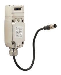
IDEM Z-Range safety switch, tongue (key) interlock, 90-degree adjustable head, (2) OSSD safety output(s), (1) status monitoring output(s), (3) status LEDs, 41 x 118 x 41mm, 316 stainless steel body, 316 stainless steel head.
