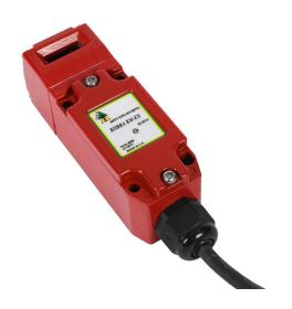
IDEM safety switch, tongue (key) interlock, hazardous location rated, 90-degree adjustable head, (2) N.C. safety output(s), (2) N.O. monitoring output(s), 40 x 118 x 43.5mm, die-cast aluminum body, die-cast aluminum head.
