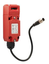
IDEM Z-Range safety switch, tongue (key) interlock, 90-degree adjustable head, (2) OSSD safety output(s), (1) status monitoring output(s), (3) status LEDs, 40 x 118 x 41mm, die-cast aluminum body, die-cast aluminum head.
