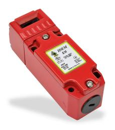
IDEM safety switch, tongue (key) interlock, 90-degree adjustable head, (2) N.C. safety output(s), (2) N.O. monitoring output(s), 40 x 118 x 41mm, die-cast aluminum body, die-cast aluminum head.
