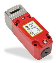
IDEM safety switch, tongue (key) interlock, 90-degree adjustable head, (2) N.C. safety output(s), (2) N.O. monitoring output(s), 40 x  $118 \times 41$ mm, die-cast aluminum body, 316 stainless steel head.
