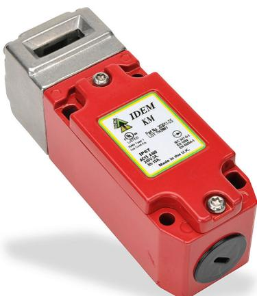
IDEM safety switch, tongue (key) interlock, 90-degree adjustable head, (2) N.C. safety output(s), (2) N.O. monitoring output(s), 40 x 118 x 41mm, die-cast aluminum body, 316 stainless steel head.
