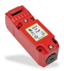
IDEM safety switch, tongue (key) interlock, 90-degree adjustable head, (3) N.C. safety output(s), (1) N.O. monitoring output(s), 40 x 118 x 41mm, die-cast aluminum body, die-cast aluminum head.
