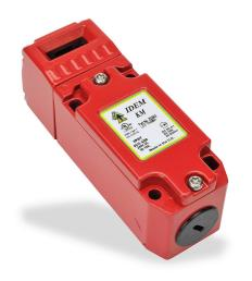
IDEM safety switch, tongue (key) interlock, 90-degree adjustable head, (2) N.C. safety output(s), (1) N.O. monitoring output(s), 40 x 118 x 41mm, die-cast aluminum body, die-cast aluminum head.
