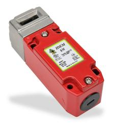
IDEM safety switch, tongue (key) interlock, 90-degree adjustable head, (2) N.C. safety output(s), (1) N.O. monitoring output(s), 40 x 118 x 41mm, die-cast aluminum body, 316 stainless steel head.
