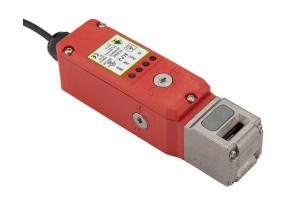
IDEM safety switch, flexible tongue (key) interlock uniquely coded RFID, solenoid, 24 VDC to unlock, 90-degree adjustable head, 2000N holding force, (2) OSSD safety output(s), (2) status monitoring output(s), polyester body, 8-pin M12 quick-disconnect.
