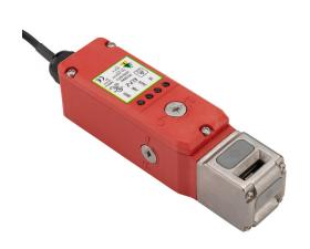
IDEM safety switch, tongue (key) interlock uniquely coded RFID, solenoid, 24 VDC to unlock, 90-degree adjustable head, 2000N holding force, (2) OSSD safety output(s), (2) status monitoring output(s), polyester body, 8-pin M12 quick-disconnect.
