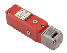
IDEM safety switch, flexible tongue (key) interlock uniquely coded RFID, solenoid, 24 VDC to unlock, 90-degree adjustable head, 2000N holding force, (2) OSSD safety output(s), (2) status monitoring output(s), polyester body, (2) 1/2in NPT cable entries.
