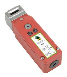
IDEM safety switch, tongue (key) interlock, solenoid, 110 VAC to unlock, 90-degree adjustable head, 1800N holding force, (2) N.C. safety output(s), (1) N.O. monitoring output(s), plastic body, (1) 1/2in NPT cable entry.
