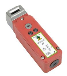
IDEM safety switch, tongue (key) interlock, solenoid, 110 VAC to unlock, 90-degree adjustable head, 1800N holding force, (2) N.C. safety output(s), (1) N.O. monitoring output(s), plastic body, (1) 1/2in NPT cable entry.
