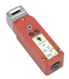
IDEM safety switch, tongue (key) interlock, solenoid, 24 VAC/VDC to unlock, 90-degree adjustable head, 1800N holding force, (2) N.C. safety output(s), (1) N.O. monitoring output(s), plastic body, (1) 1/2in NPT cable entry.
