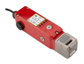
IDEM safety switch, flexible tongue (key) interlock uniquely coded RFID, solenoid, 24 VDC to unlock, 90-degree adjustable head, 3000N holding force, (2) OSSD safety output(s), (2) status monitoring output(s), die-cast aluminum body, 8-pin M12 quickdisconnect.
