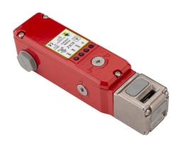
IDEM safety switch, flexible tongue (key) interlock uniquely coded RFID, solenoid, 24 VDC to unlock, 90-degree adjustable head, 3000N holding force, (2) OSSD safety output(s), (2) status monitoring output(s), die-cast aluminum body, (2) 1/2in NPT cable entries.
