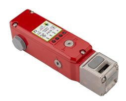
IDEM safety switch, tongue (key) interlock uniquely coded RFID, solenoid, 24 VDC to unlock, 90-degree adjustable head, 3000N holding force, (2) OSSD safety output(s), (2) status monitoring output(s), die-cast aluminum body, (2) 1/2in NPT cable entries.
