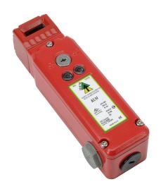
IDEM safety switch, tongue (key) interlock, solenoid, 110 VAC to unlock, 90-degree adjustable head, 2000N holding force, (4) N.C. safety output(s), (1) N.O. monitoring output(s), die-cast aluminum body, (3) 1/2in NPT cable entries.
