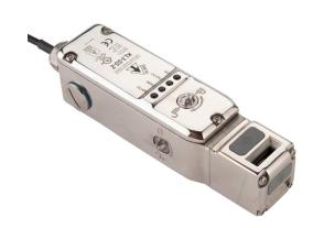
IDEM safety switch, flexible tongue (key) interlock uniquely coded RFID, solenoid, 24 VDC to unlock, 90-degree adjustable head, 3000N holding force, (2) OSSD safety output(s), (2) status monitoring output(s), 316 stainless steel body.
