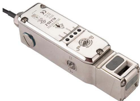
IDEM safety switch, flexible tongue (key) interlock uniquely coded RFID, solenoid, 24 VDC to unlock, 90-degree adjustable head, 3000N holding force, (2) OSSD safety output(s), (2) status monitoring output(s), 316 stainless steel body.
