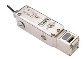
IDEM safety switch, tongue (key) interlock uniquely coded RFID, solenoid, 24 VDC to unlock, 90-degree adjustable head, 3000N holding force, (2) OSSD safety output(s), (2) status monitoring output(s), 316 stainless steel body, 8-pin M12 quick-disconnect.
