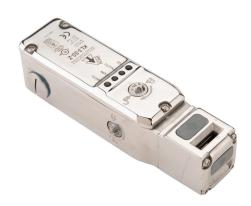
IDEM safety switch, flexible tongue (key) interlock uniquely coded RFID, solenoid, 24 VDC to unlock, 90-degree adjustable head, 3000N holding force, (2) OSSD safety output(s), (2) status monitoring output(s), 316 stainless steel body.
