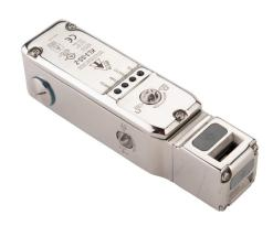
IDEM safety switch, tongue (key) interlock uniquely coded RFID, solenoid, 24 VDC to unlock, 90-degree adjustable head, 3000N holding force, (2) OSSD safety output(s), (2) status monitoring output(s), 316 stainless steel body, (2) 1/2in NPT cable entries.
