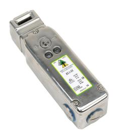
IDEM safety switch, tongue (key) interlock, solenoid, 110 VAC to unlock, 90-degree adjustable head, 2000N holding force, (4) N.C. safety output(s), (1) N.O. monitoring output(s), 316 stainless steel body, (3) 1/2in NPT cable entries.
