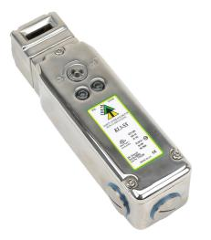
IDEM safety switch, tongue (key) interlock, solenoid, 24 VAC/VDC to unlock, 90-degree adjustable head, 2000N holding force, (4) N.C. safety output(s), (1) N.O. monitoring output(s), 316 stainless steel body, (3) 1/2in NPT cable entries.
