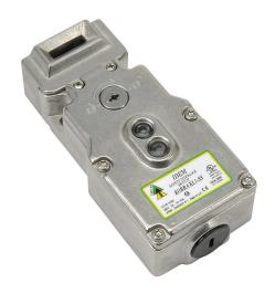
IDEM safety switch, tongue (key) interlock, solenoid, 24 VAC/VDC to unlock, 180-degree adjustable head, 1600N holding force, (2) N.C. safety output(s), (1) N.O. monitoring output(s), 316 stainless steel body, (1) 1/2in NPT cable entry.
