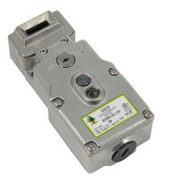
IDEM safety switch, tongue (key) interlock, solenoid, 110 VAC to unlock, 180-degree adjustable head, 1600N holding force, (2) N.C. safety output(s), (2) N.O. monitoring output(s), 316 stainless steel body, (1) 1/2in NPT cable entry.
