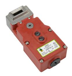
IDEM safety switch, tongue (key) interlock, solenoid, 110 VAC to unlock, 180-degree adjustable head, 1400N holding force, (2) N.C. safety output(s), (1) N.O. monitoring output(s), plastic body, (1) 1/2in NPT cable entry.
