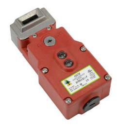
IDEM safety switch, tongue (key) interlock, solenoid, 24 VAC/VDC to unlock, 180-degree adjustable head, 1400N holding force, (2) N.C. safety output(s), (1) N.O. monitoring output(s), plastic body, (1) 1/2in NPT cable entry.
