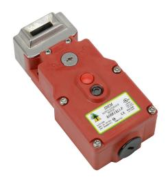
IDEM safety switch, tongue (key) interlock, solenoid, 110 VAC to unlock, 180-degree adjustable head, 1400N holding force, (2) N.C. safety output(s), (2) N.O. monitoring output(s), plastic body, (1) 1/2in NPT cable entry.
