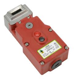
IDEM safety switch, tongue (key) interlock, solenoid, 24 VAC/VDC to unlock, 180-degree adjustable head, 1400N holding force, (2) N.C. safety output(s), (2) N.O. monitoring output(s), plastic body, (1) 1/2in NPT cable entry.
