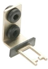
Comepi actuator tongue (key), shock absorbing, 90 degree mounting tab with 15mm mounting hole spacing mount, 316 stainless steel. For use with Comepi SP2K and SDM2K series safety switches.
