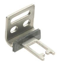
Comepi actuator tongue (key), 90 degree mounting tab with 13mm mounting hole spacing mount, 316 stainless steel. For use with Comepi SP2K and SDM2K series safety switches.
